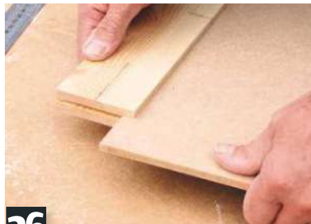
26 Check panel is sliding fit in groove without being too tight. Depth should be about 10mm
